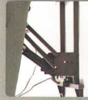
Altering the pin position on both sides of the action changes the angle of rise
